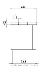
Measurements are in millimetres. Drawings are not to scale. Dimensions show are for timber slat option.
